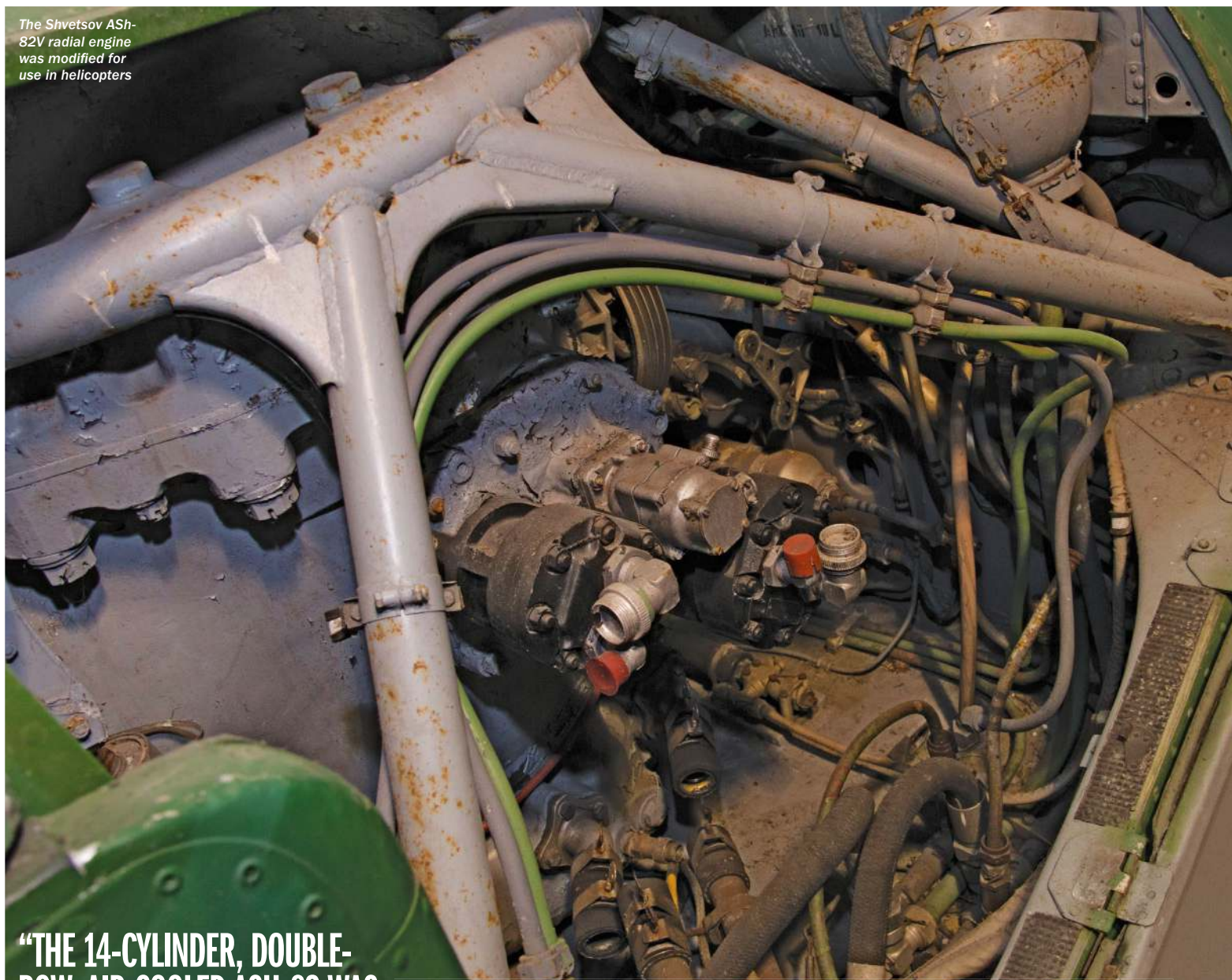
The powerplant and rotor system of the Mi-4 delivers 1,675 horsepower and provides a moderate cruising speed
